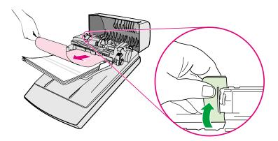
If the item cannot be easily removed, lift the two green tabs located behind the rollers and gently remove the green paper lead as shown.
